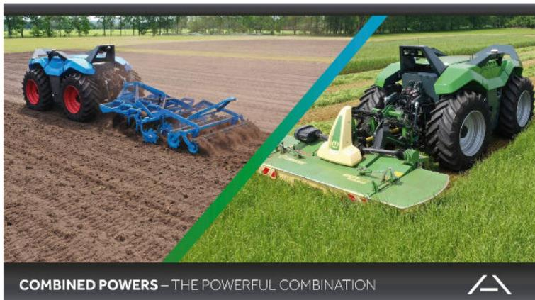
High-performance electrification: The process unit from KRONE and LEMKEN uses high-performance motors and other components from the modular eLION platform in order to perform a wide range of work processes in the optimum manner. (Image source: Maschinenfabrik Bernard KRONE GmbH & Co. KG)
