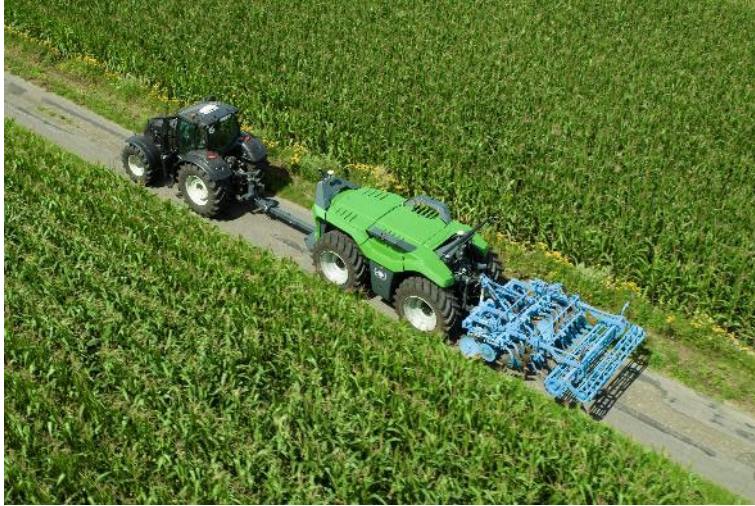
Fig. 1: The Vehicle Transport System (VTS) from Krone and Lemken enables transport by tractor.
