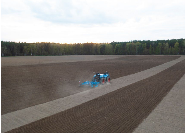
Fig.1: Combined Powers in use at LEMKEN: A mounted cultivator Karat is cultivator is used as a smart implement with sensor control.
