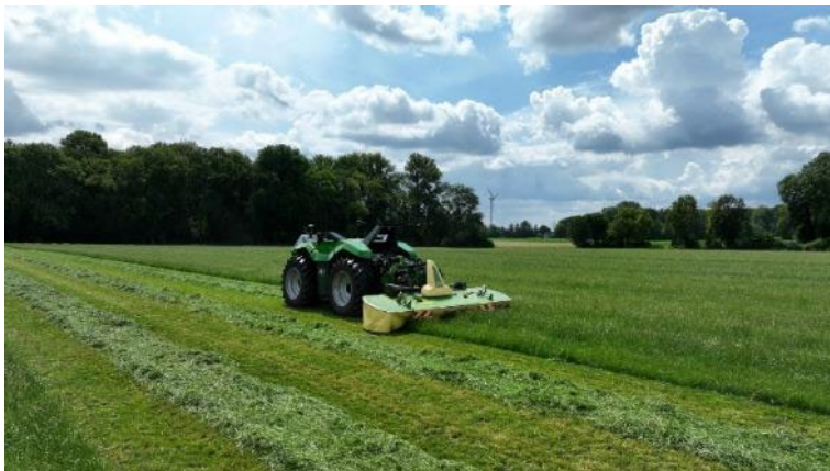
Fig. 1: Combined Powers in use at KRONE: A front disc mower is used as a smart implement.
