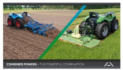
High-performance electrification: The process unit from KRONE and LEMKEN uses high-performance motors and other components from the modular eLION platform in order to perform a wide range of work processes in the optimum manner. (Image source: Maschinenfabrik Bernard KRONE GmbH & Co. KG)
